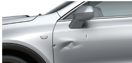
Hail damage or punctures on any panel
