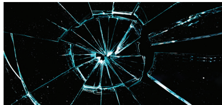
Cracked glass greater than 1/2” in diameter or spidered cracks
