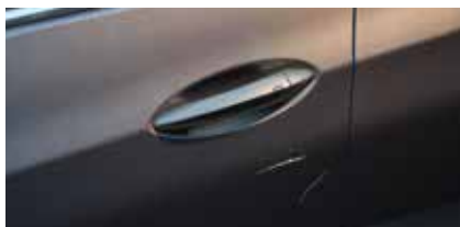
1 dent or 2 scratches (less than 4”) per panel
