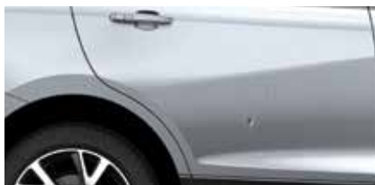
Fewer than 4 dings (less than 2”) per panel
