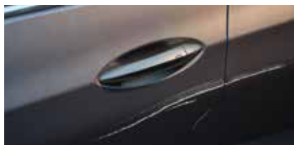
1 dent or 2 scratches (more than 4”) per panel
