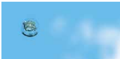
Cracked glass less than 1/2” in diameter
