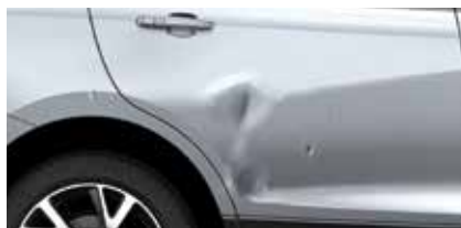
Hail damage or punctures on any panel
