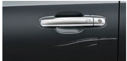
1 dent (more than 4") or 1 scratch (equal to or more than 6") per panel
