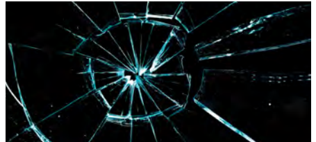
Cracked glass (equal to or more than 1/2" in diameter) or spidered cracks
