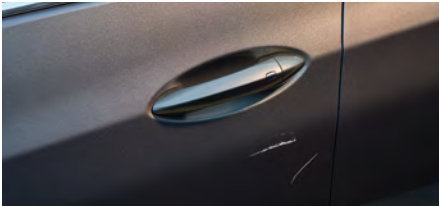
1 dent (equal to or less than 4") or 1 scratch (less than 6") per panel
